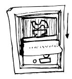
A rubber squeegee is used to spread a thin layer of ink evenly across the screen.
