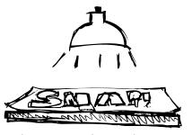
Light causes a chemical reaction, bonding the chemicals to the exposed parts of the screen.
