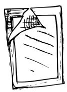
A fine mesh screen is stretched around a frame.
