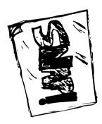
A positive is made by drawing or printing a design on transparent material.
